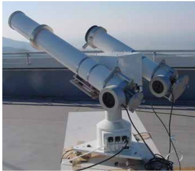
Photo 1 View of the collimation tube with pyranometer. The pyranometer without sunscreen is attached to the bottom of the tube.
