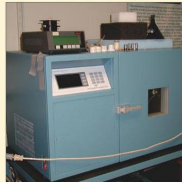
Figure 5: Humidity calibration chamber at the WHOI calibration facility.
