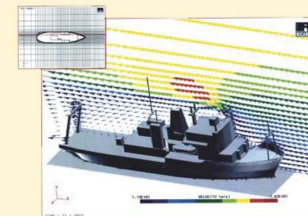
Figure 9: Flow field from the Southampton Oceanography Centre computational fluid dynamics model for the Research Vessel Darwin.
