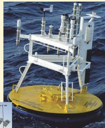
Figure 1 (above): The Northwest Tropical Atlantic Station (NTAS) buoy with ASIMET modules. Figure 2 (inset): Close-up of ASIMET modules on NTAS buoy tower.
