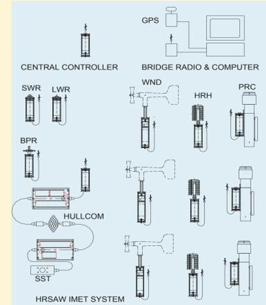
Figure 8: Block diagram of portable, wireless ASIMET system.
