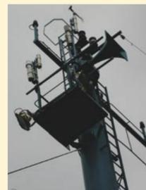
Figure 3 (above): The VOS Sea-Land Enterprise at sea. Figure 4 (right): Bow mast of the VOS Columbus Florida with first-generation ASIMET modules installed.
