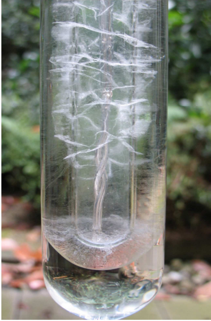
Figure 3. Triple point of water cell and SPRT
