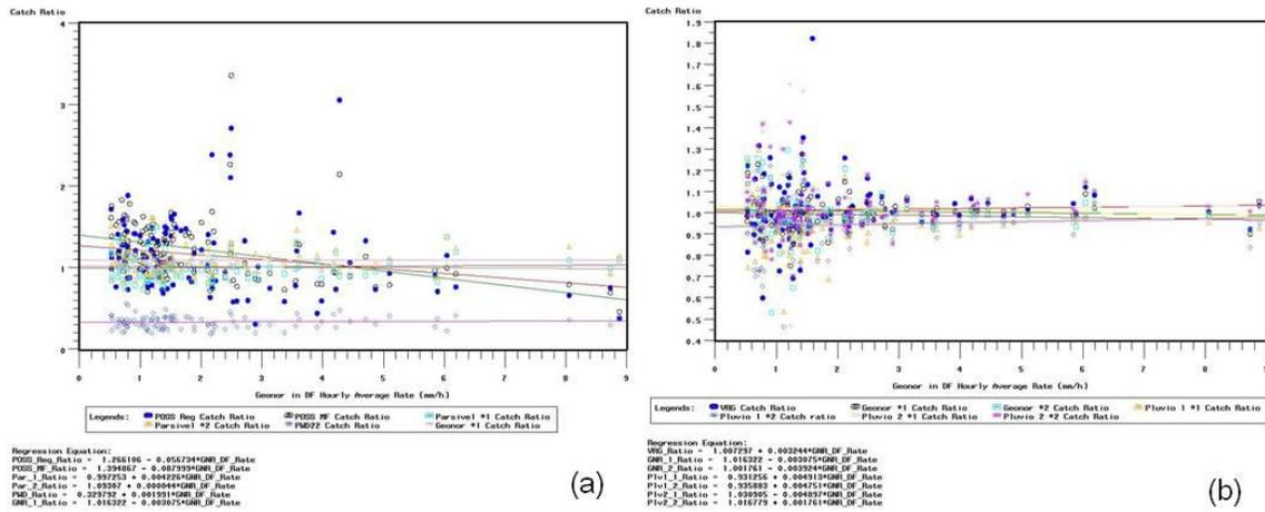
**Figure 10 – (a) Catch ratios of the present weather sensors vs. hourly precipitation rates of the Geonor in DF for liquid precipitation, and (b) Catch ratios of the precipitation gauges vs. hourly precipitation rates of the Geonor in DF for liquid precipitation.**
