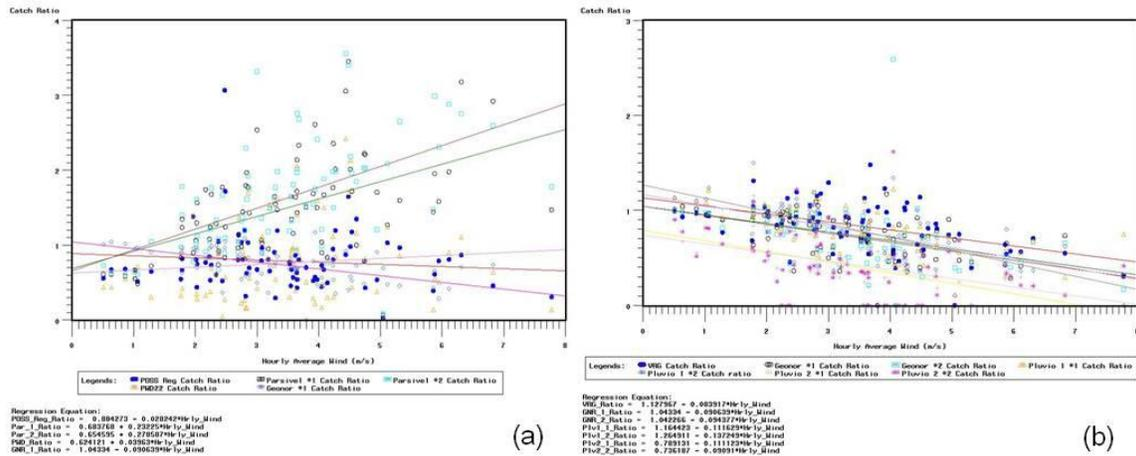
**Figure 13 – (a) Catch ratios of the present weather sensors vs. hourly average winds for solid precipitation, and (b) Catch ratios of the precipitation gauges vs. hourly average winds for solid precipitation.**
