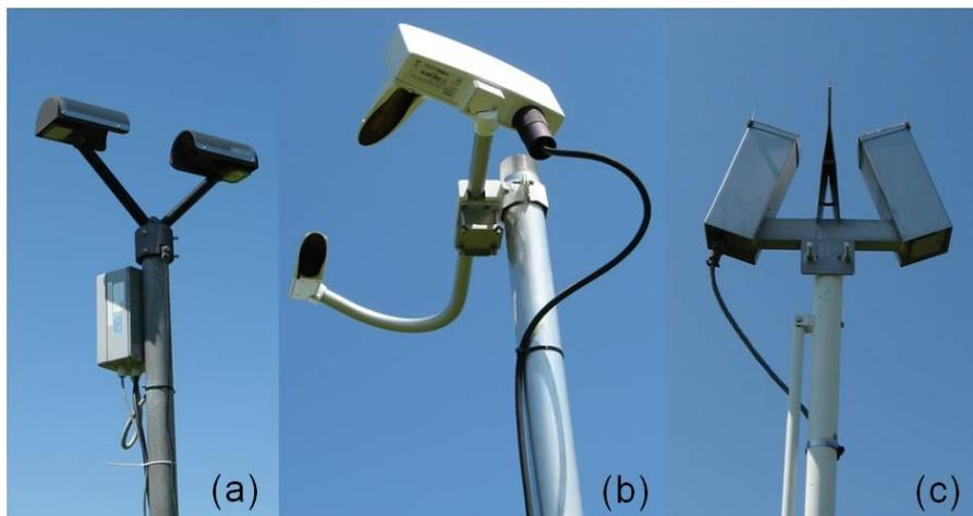
Figure 2 – OTT Parsivel present weather sensor (a), Vaisala PWD22 present weather detector (b), Qualimetrics/AWI POSS (C).
