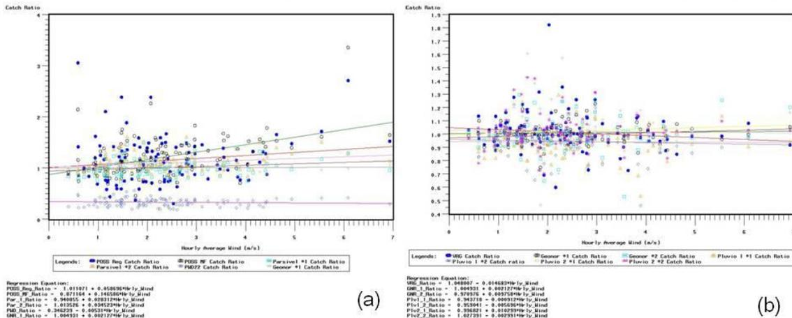
**Figure 8 – (a) Catch ratios of the present weather sensors vs. hourly average winds for liquid precipitation, and (b) catch ratios of the precipitation gauges vs. hourly average winds for liquid precipitation.**
