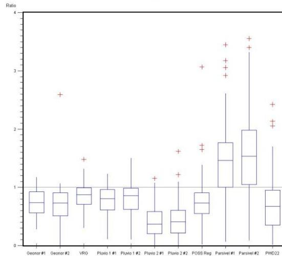
Figure 11 - Catch ratios of hourly amounts for solid precipitation.
