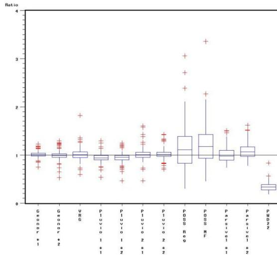
Figure 6 - Catch ratios of hourly amounts for liquid precipitation.
