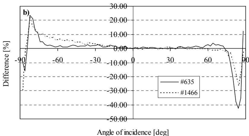
Figure 1. Deviation of the angular response from the ideal cosine response for the two SL 501 radiometers as measured at STUK during the WMO/STUK '95 intercomparison and in 1999 (a), percentage deviation between the measurements by STUK in 1995 and 1999 (b).
