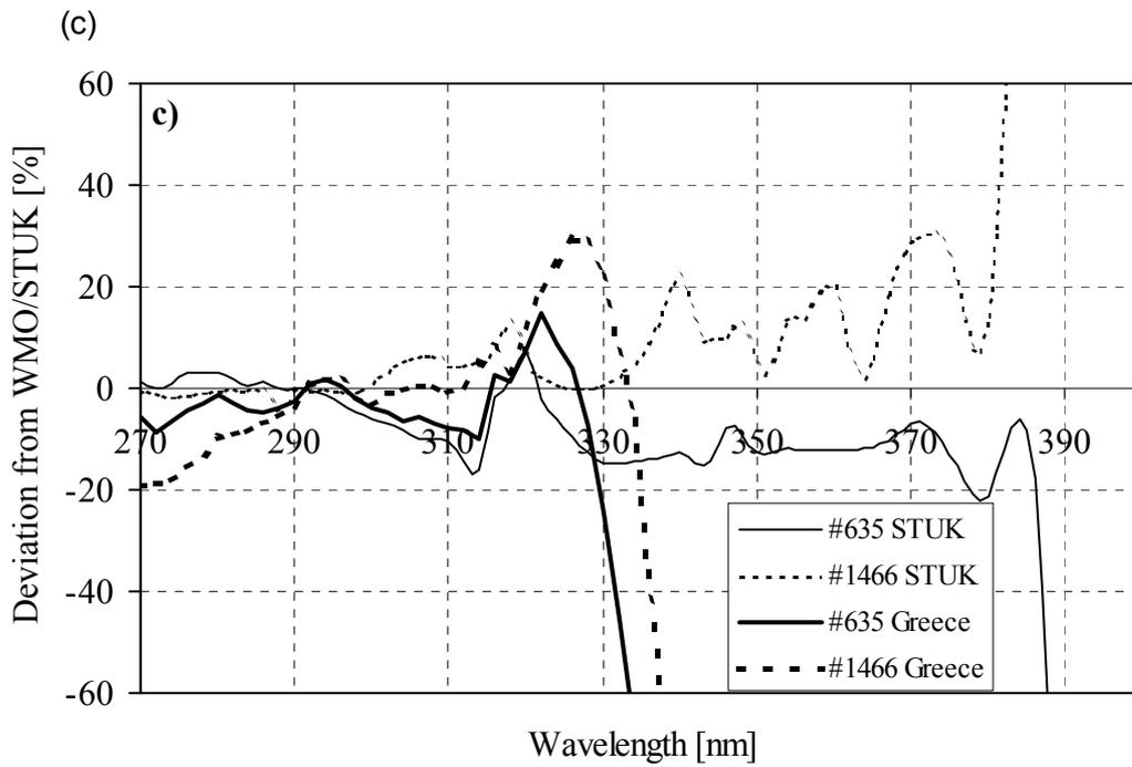
**Figure 2.** Spectral responsivities of the SL 501 meters # 635 (a) and #1466 (b) as measured during WMO/STUK '95 intercomparison and in 1999 by STUK, and UTH (Bais et al. 2000). (c) Percentage deviations of the 1999 results from the WMO/STUK '95 intercomparison data.
