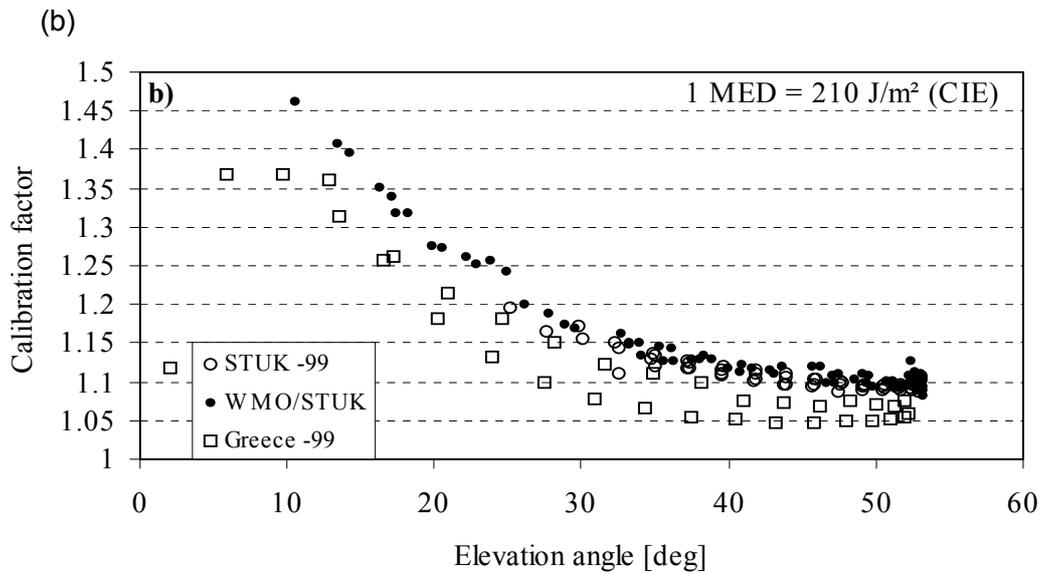
**Figure 3.** Calibration factors (CF's) of the SL 501 # 635 (a) and # 1466 (b) as a function for solar elevation angle obtained at STUK in Finland in 1995 and in 1999, and in Greece in 1999 (Bais et al. 2000).
