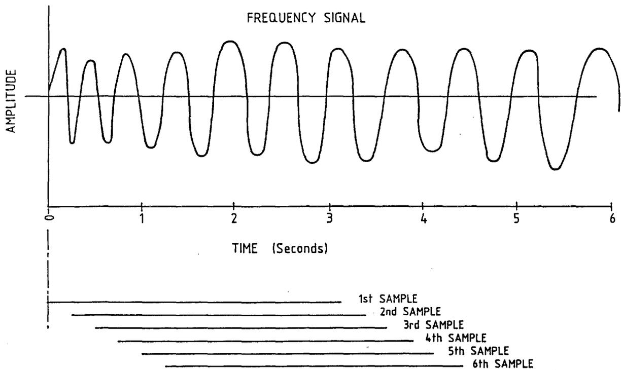
Figure 2. FREQUENCY INPUT SAMPLING.
