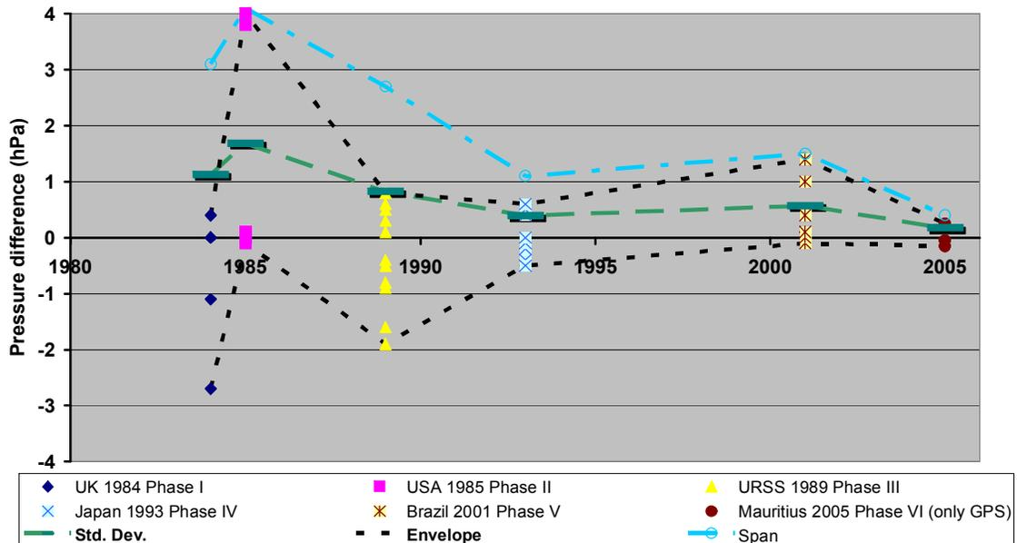
**Figure 12.** Bias of the pressure measurements and/or derivations around 100 hPa for the six WMO Radiosonde Comparisons (simultaneous measurements). The two dotted lines represent the envelope of all individual results, which is converted into a span with the dash-dotted line. The horizontal green bars on the dashed green curve correspond to one standard deviation of the biases for each comparison.
