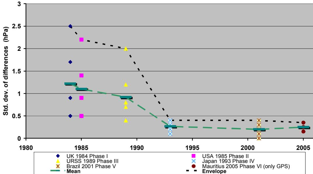
**Figure 13.** Estimated random errors of the pressure measurements and or derivations around 100 hPa for the six WMO Radiosonde Comparisons (simultaneous measurements). The dotted line represents the envelope of all individual results. The horizontal green bars on the dashed green curve correspond to the mean random errors.
