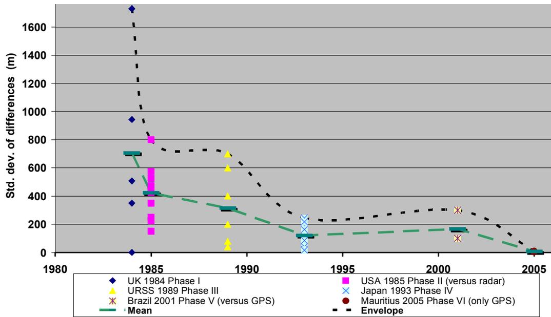
**Figure 8.** Estimated random errors of the geopotential height measurements around 10 hPa for the six WMO Radiosonde Comparisons (simultaneous measurements). The dotted line represents the envelope of all individual results. The horizontal green bars on the dashed green curve correspond to the mean random errors.
