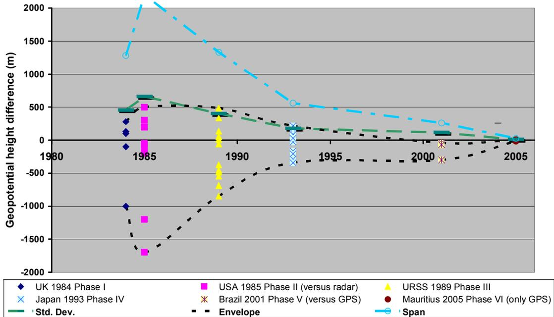
**Figure 7.** Bias of the geopotential altitude around 10 hPa for the six WMO Radiosonde Comparisons (simultaneous measurements). The two dotted lines represent the envelope of all individual results, which is converted into a span with the dash-dotted line. The horizontal green bars on the dashed green curve correspond to one standard deviation of the biases for each comparison.
