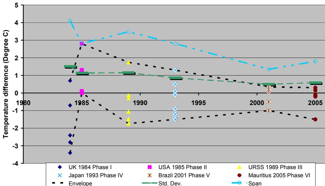
**Figure 5.** Night-time temperature bias around 10 hPa for the six WMO Radiosonde Comparisons (simultaneous measurements). The two dotted lines represent the envelope of all individual results, which is converted into a span with the dash-dotted line. The
