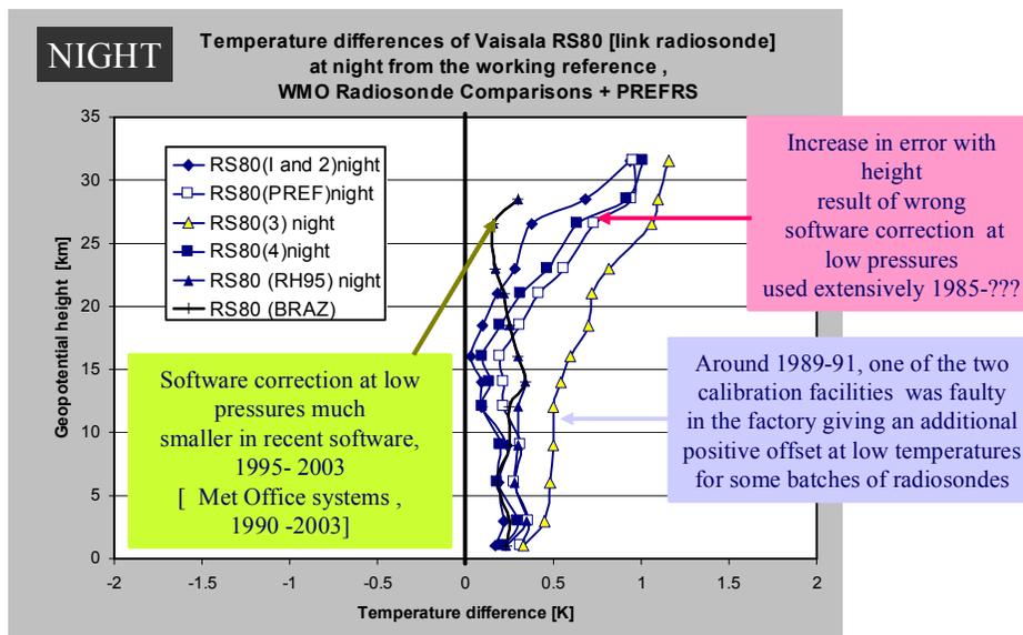
Figure 11. Range of systematic errors in RS80 temperature measurements from 1984 to 2003 [Nash, 2004].
