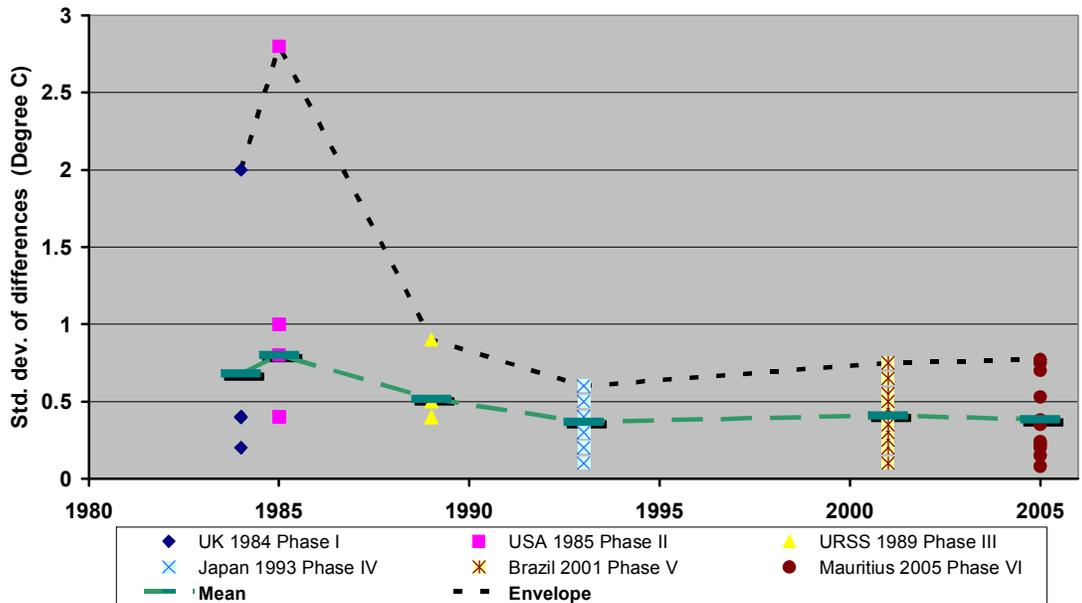
**Figure 10.** Estimated random errors of the temperature measurements around 10 hPa for the six WMO Radiosonde Comparisons (simultaneous measurements). The dotted line represents the envelope of all individual results. The horizontal green bars on the dashed green curve correspond to the mean random errors.
