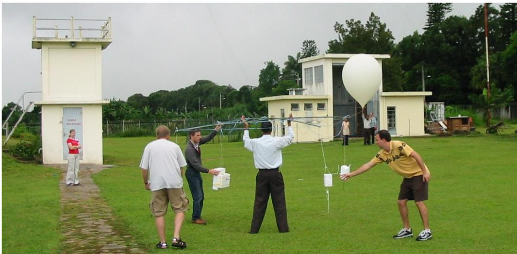
**Figure 4.** Radiosondes launch during the WMO Radiosonde Comparison at Vacaos, Mauritius, 2005.
