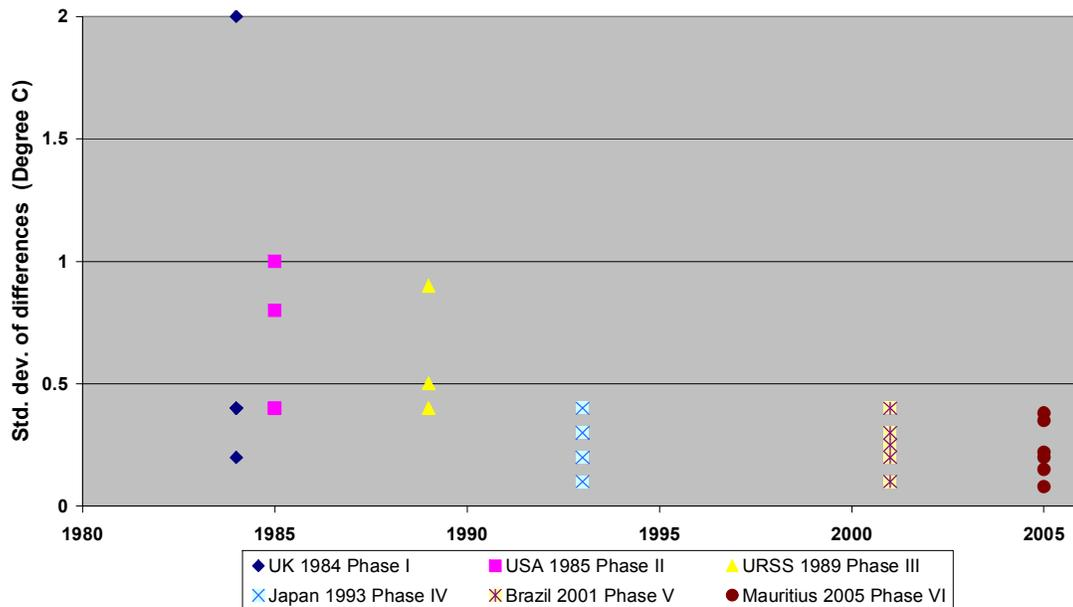
**Figure 6.** Estimated random errors of the night-time temperatures around 10 hPa for the six WMO Radiosonde Comparisons (simultaneous measurements).
