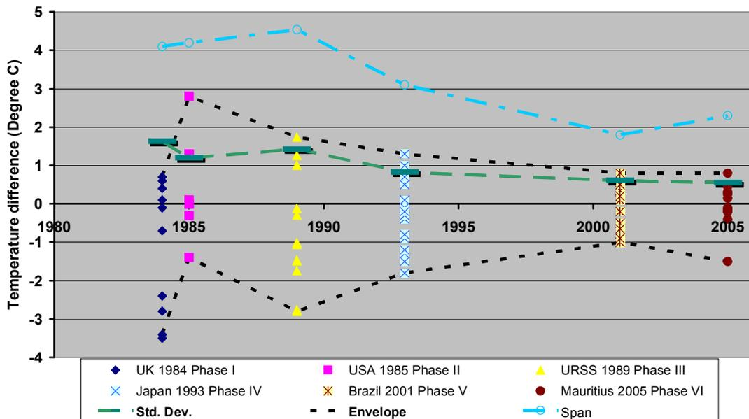
**Figure 9.** Night and day time temperature bias around 10 hPa for the six WMO Radiosonde Comparisons (simultaneous measurements). The two dotted lines represent the envelope of all individual results, which is converted into a span with the dash-dotted line. The horizontal green bars on the green dashed curve correspond to one standard deviation of the biases of each comparison.
