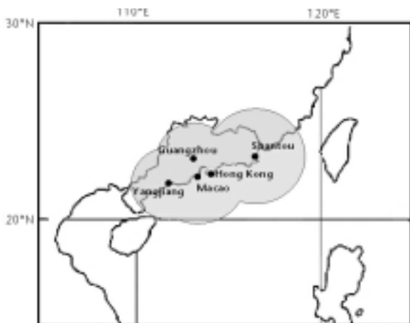
Figure 2(b)—Exchange of radar data among Guangdong Province, Macao and Hong Kong commenced in 2002. The shaded area denotes combined coverage of the weather radar.
