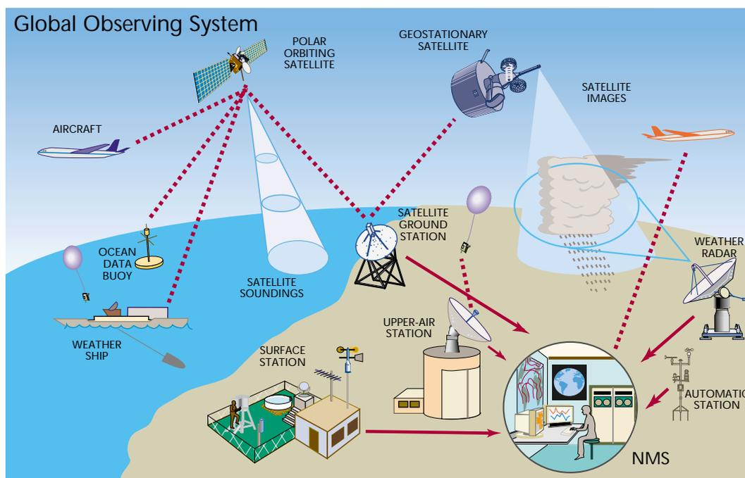
A variety of instruments on the land, oceans, aircraft and in space are used to measure characteristics of the atmosphere and the oceans and to monitor weather systems.
