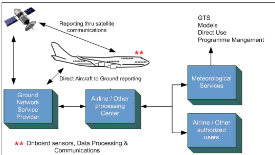
Figure 1: The AMDAR observing system.
