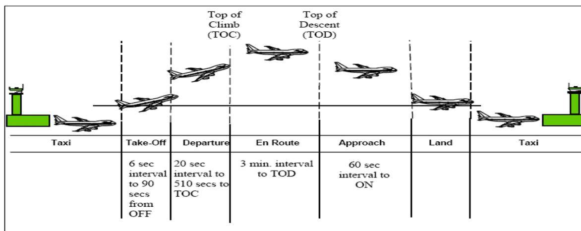
Figure 2: Reporting of AMDAR Observations during the different phases of flight (based on a particular configuration of the AEEC ARINC 620 Meteorological Report time-based specification).
