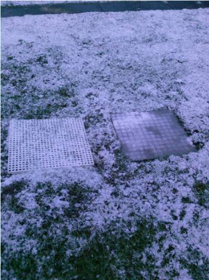
Figure: German snow plate (right) for use with automatic snow depth sensors, ultrasonic type.
