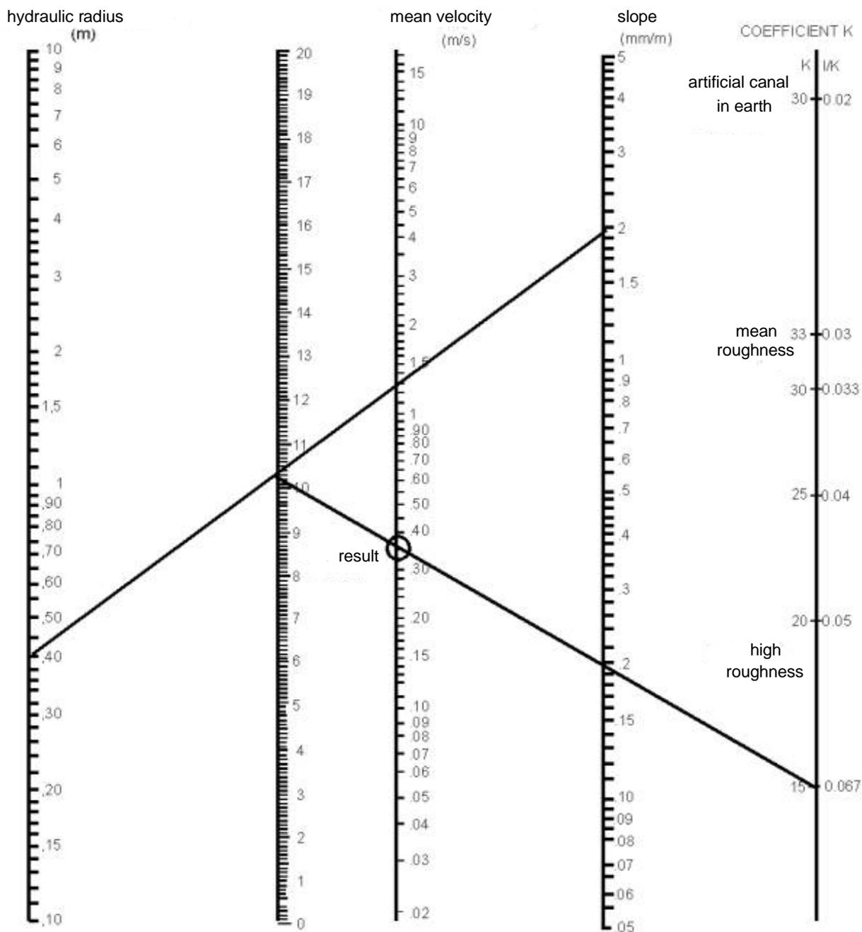
Exemple :  $R = 0.4 \text{ m}$   $J = 2 \text{ mm/m}$   $K = 15 \Rightarrow U = 0.36 \text{ m/s}$
