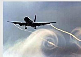
Visualization of wake vortices generated by an aircraft by clouds
