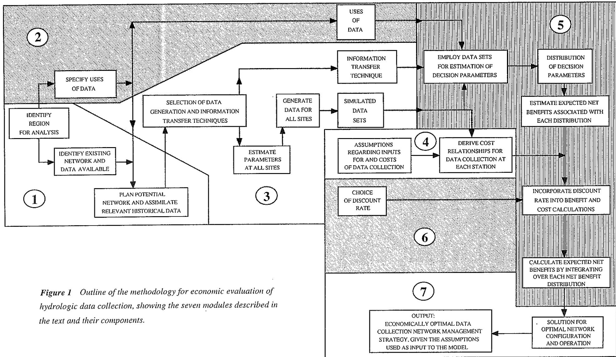
Figure 1 Outline of the methodology for economic evaluation of hydrologic data collection, showing the seven modules described in the text and their components.
