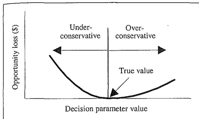
Figure 2 Conceptual representation of relationship between decision parameter error and opportunity loss (cost of errors).
